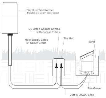
Coil leftover lead wire at base of luminaire inside installation tube.
