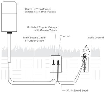
Coil leftover lead wire at base of luminaire.
